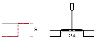
24 LINEAR REGULAR - T24 ribassato/lowered 15mm
