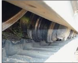
De-tracking at track roller
