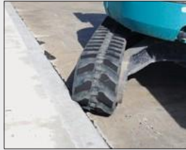
Common cause of edge-cut
