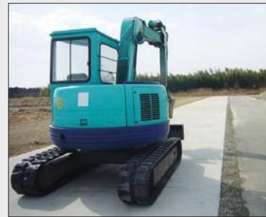
Testing carried out at Bridgestone's proving ground in Tochigi Japan using 5.3ton machine on asphalt.
