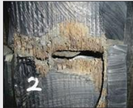
Steel cord deterioration caused by rust
