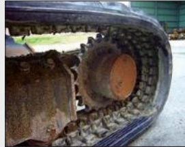
De-tracking at sprocket
