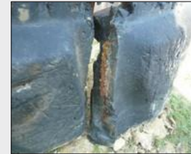
Steel cord deterioration caused by rust
