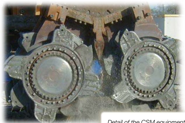
Detail of the CSM equipment
