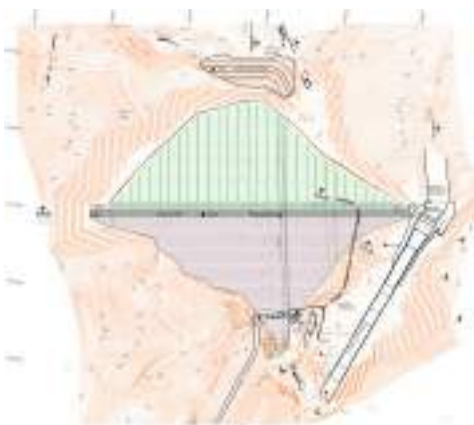
Layout of the works of Misicuni Dam
